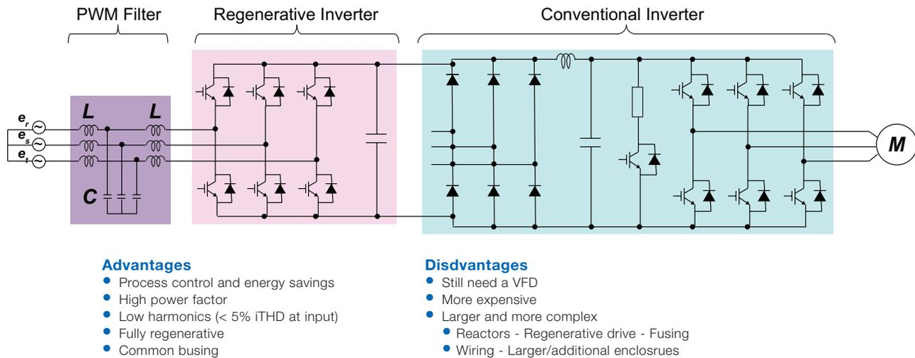
An AFE saves energy by putting the regenerative energy back onto the line. However, unlike an FFE, an AFE uses a PWM waveform to regenerate back onto the line.
