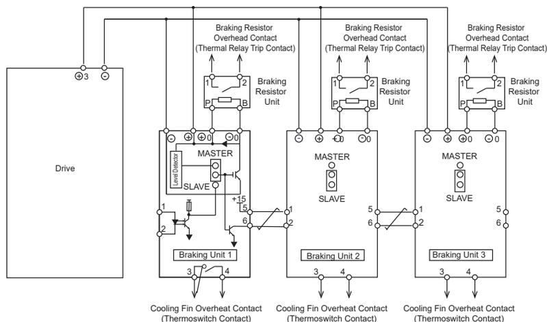
Drive with Internal Braking Switches
